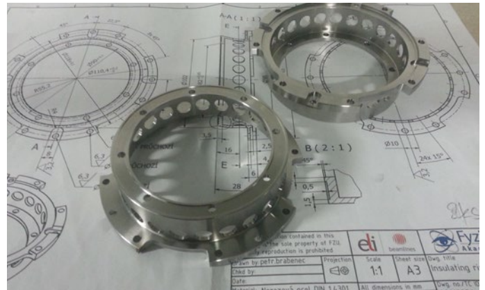
Beam dump - parts (L1 laser system).
