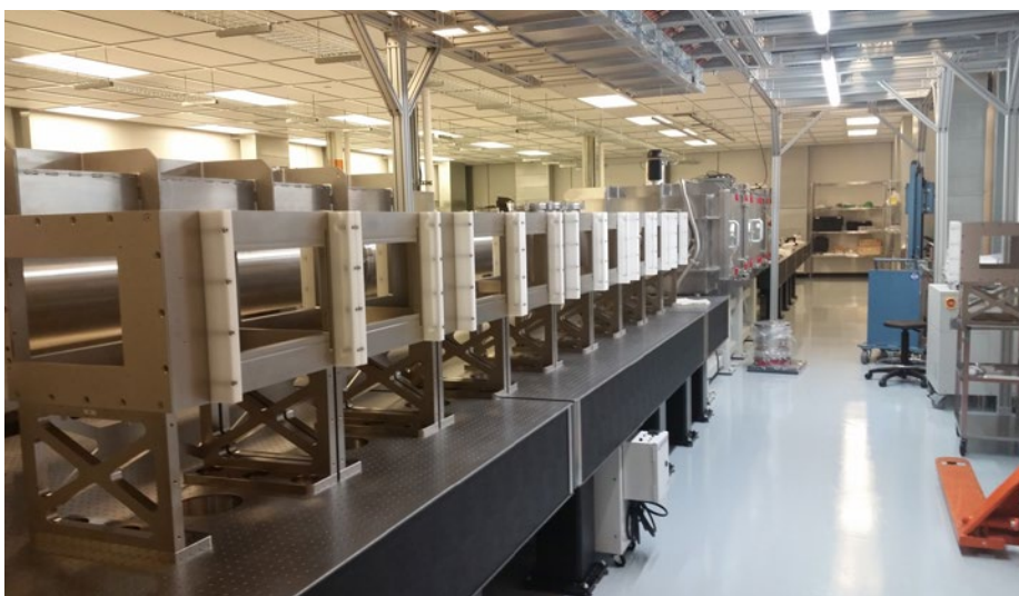
The assembly of Nd:glass Power Amplifier 1.
